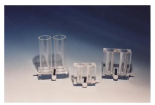
PHERO-grad gradient mixer is supplied as standard to ensure efficient gradient formation by mixing and delivering high- and low-density denaturant solutions. A flat-base design and support handle allows the PHERO-grad to be secured to a retort stand, enabling it to be easily mounted on a magnetic stirring plate, while the mixing chamber can accommodate a magnetic stirrer to form a linear gradient. A peristaltic pump is also recommended for delivery of linear and reproducible gradient gels.
