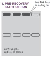
1. Load sample in 'loading tier' of wells.
