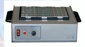
Temperature setting: analog Temperatur range: RT.. 105°C
