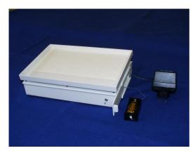
PHERO shaker mini is the ideal instrument to be used in your lab wherever you want. The table size of  $29 \times 19$  cm offers the use for shaking of every standard sized gel. Because it comes with battery you can work independent from every power line. This gives the advantage of using this instrument inside of e.g. refridgerators or incubators.
