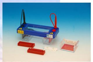
The PHERO-sub 0710 E is the smallest unit in the range, designed for low to medium numbers of samples. The small gel size maximises run economy but does not compromise versatility as two tray options are available –  $7 \times 7$ cm and  $7 \times 10$ cm, and combs ranging from preparative up to 16 samples. Simply by altering the gel tray or comb, this compact unit is capable of resolving up to 64 different samples, prepping 1ml of sample or separating sample bands over a distance of 9cm.
