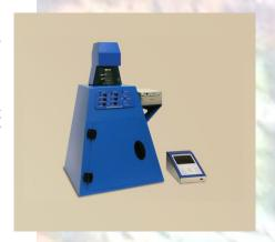
142214-001 Gel Documentation system Gerix 1040 (CCD Camera, Cabinet, UV-Transilluminator, Control unit)
