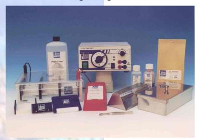
This workstation is based on manual electrophoresis tank modell 1000 and contains all equipment to run electrophoresis on agarose gel
